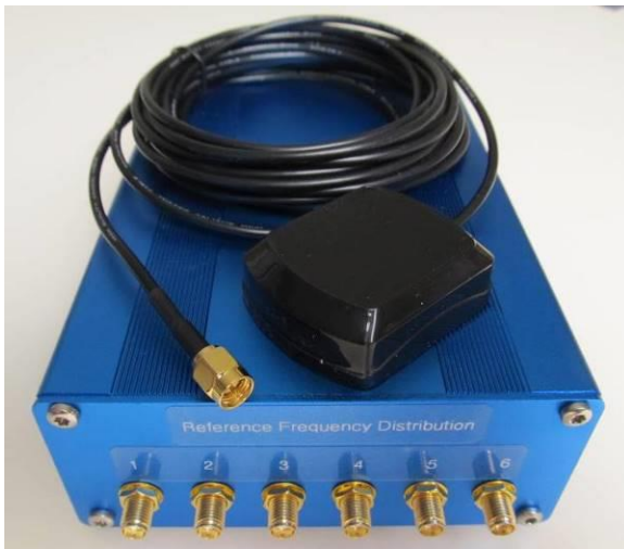
Figure 1 ~ Front view of the Reference Frequency Distribution System showing the six outputs and an optional GPS antenna resting on top. The rear panel, not seen here, holds the reference or GPS antenna input, an On-Off switch, power indicating LED and coaxial dc power jack. The enclosure dimensions are 1.77H x 4.27W x 6.30L in (45 x 108.5 x 160 mm) and weight is 1 lb (0.5 kg). Image ©2020 W. Reeve
