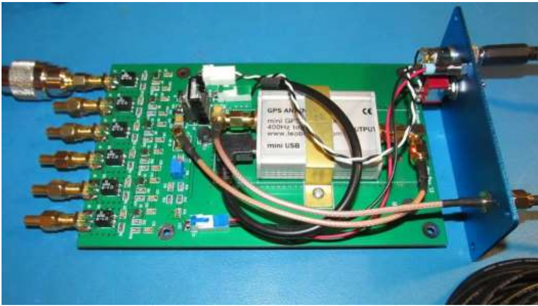
Figure 5 ~ Prototype of the Reference Frequency Distribution System with rear panel while under test. The SMA-F connectors for the six outputs are seen on the left edge of the PCB; channel 1 (upper-left) is connected to the spectrum analyzer for measurements and channels 2 – 6 have 50 ohm terminations. The output transformers are immediately to the right of the RF connectors, and the six identical amplifier circuits are to the right of the transformers. All components are grouped so that the PCB may be cut down and used in a shorter enclosure if the Mini-GPS Reference Clock is not equipped. It is shown here mounted with a metal strap (see text). The power and LED interfaces use friction lock connectors. The prototypes used an MCX-F socket on the PCB (seen here just to the left of the Mini-GPS Reference Clock antenna connection) for connecting the reference source input. This connector was replaced with an SMA-F connector in the production versions. Image ©2020 W. Reeve
