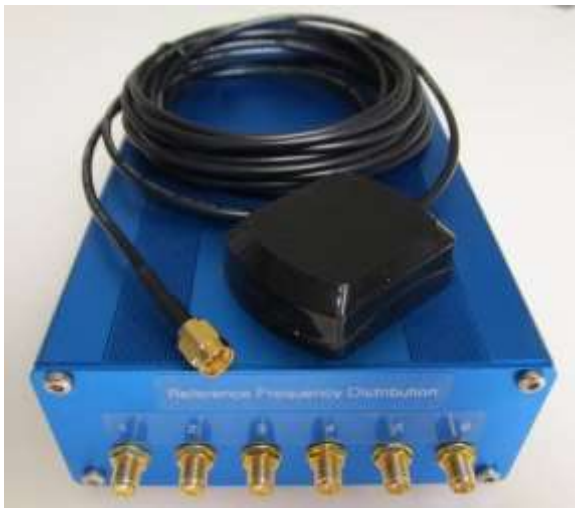
Figure 1 ~ Front view of the Reference Frequency Distribution System showing the six outputs and an optional GPS antenna resting on top. The rear panel, not seen here, holds the reference or GPS antenna input, an On-Off switch, power indicating LED and coaxial dc power jack. The enclosure dimensions are 1.77H x 4.27W x 6.30L in (45 x 108.5 x 160 mm) and weight is 1 lb (0.5 kg). Image ©2020 W. Reeve
