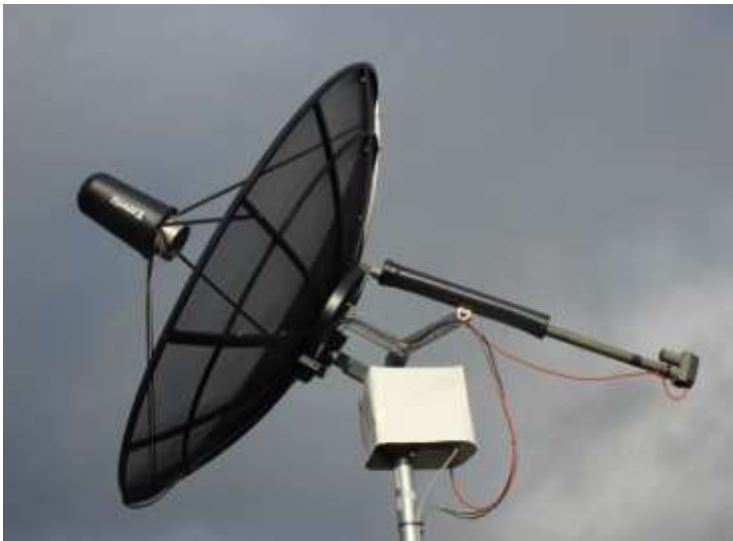
Figure 1: 2.3-m dish used for the observation
