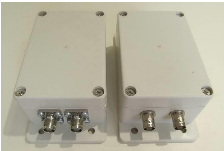
Figure 8 ~ Completed units ready for final testing, BNC on the left and TNC on the right. ©2020 W. Reeve
