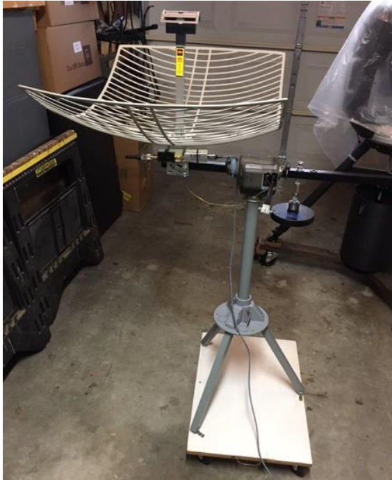
Figure 3 – Motor with antenna on one side and counterweight on the other. Tripod is braced on board with wheel casters.
