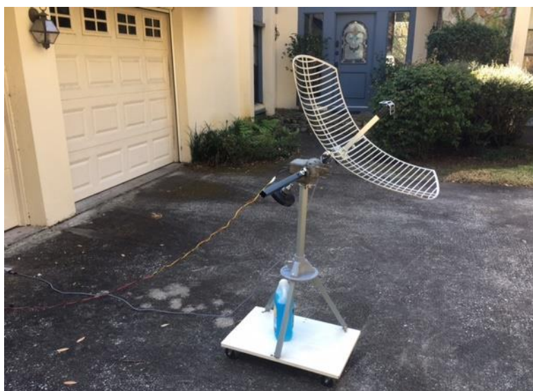
Figure 5 – Antenna outdoors operated via two 10 ft USB3 cables in series.
