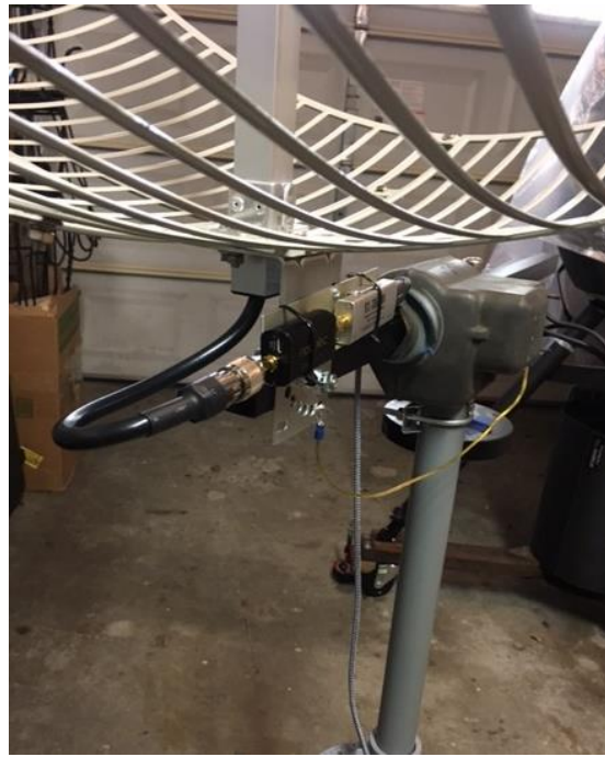
Figure 4 – Coax twisted once to meet LNA- SDR tandem, attached with zip ties near to rotation axis so USB cable gets minimal torsion when motor rotates.
