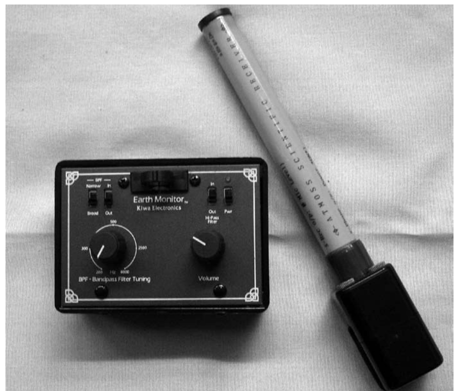
Figure 3 — This photo shows the Kiwa Earth Monitor (left) and Brian Lucas' ATMOSS (right) VLF receivers. (Photo by author.)
