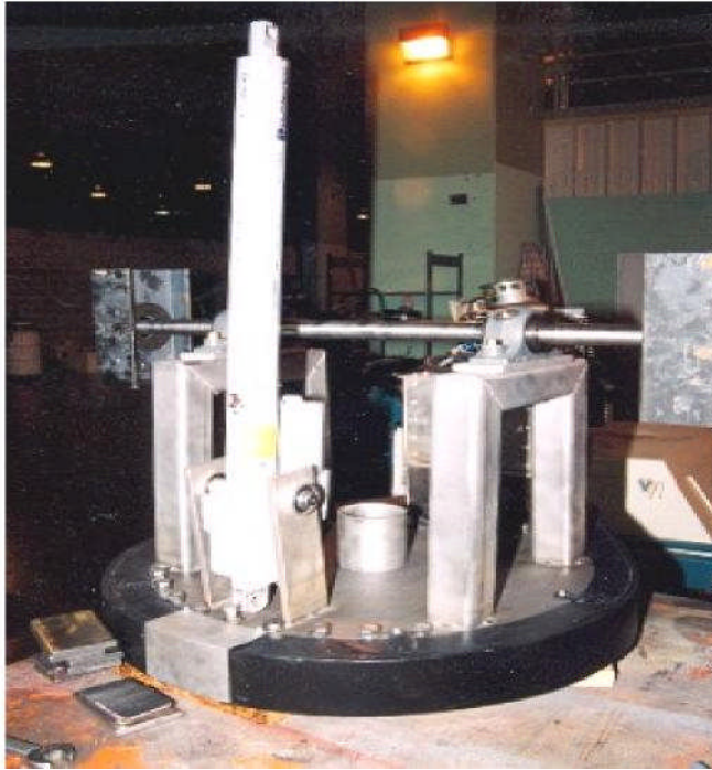
Fig. 7 – The U-frame shaft supports are welded to the 1 in upper support plate. On top of the U-frames is the support shaft for the 2 in diameter dish arms. The vertical actuator ram (vertical shaft on left) is mounted on two 1/2 in x 3 in plates welded to the upper 1 in support plate. The ram pivots are mounted in 1 in sealed needle bearings. Needle bearings can carry a high load for their size.
