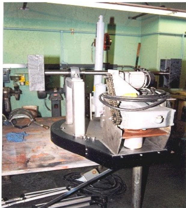
Fig. 8 – Rotor set up for testing. A sheet metal dust cover at bottom of the assembly is covering the thrust bearing gear teeth to lessen dust getting into the heavy grease that coats the gear teeth and to keep snow and ice out of the teeth. The coil of cable on the worm gear torque box is for testing and not used in the finished rotor. The dish supports and counterweight arms bolt to short I-beam sections on either side of the horizontal shaft. A 1/4 hp azimuth drive motor is mounted on top of the worm gear torque box and drives it through a chain drive. The worm gear drive and bull gear can handle 18,000 ft-lb of torque.
