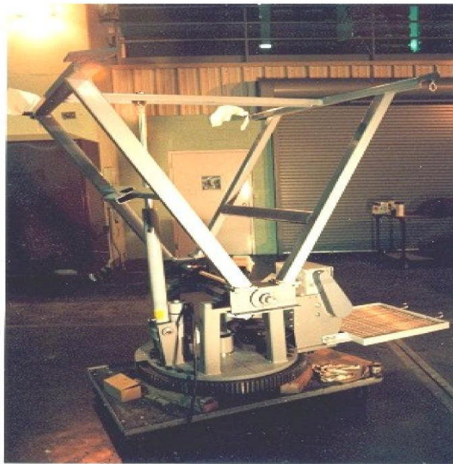
Fig. 4 – A-frame dish support shown in vertical position with the vertical actuator ram fully extended. Also shown is the I-beam coupling of the A-frame to support shaft. The counterweight arms are attached to back side of the I-beam. The work platform shown at lower-right behind the azimuth drive was awfully small when the rotor was mounted on the pole and the wind was blowing.
