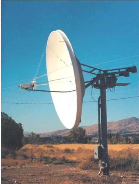
Fig. 10. – IT IS DONE! The 24 ft dish antenna on its support poles with the rotor system and associated structure
