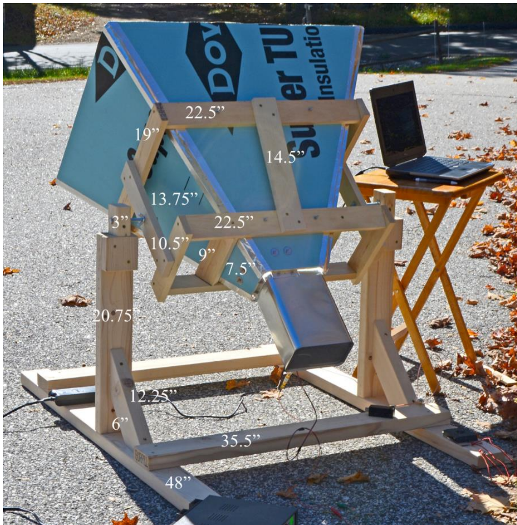
Figure 6: Horn with Stand Including Measurements
