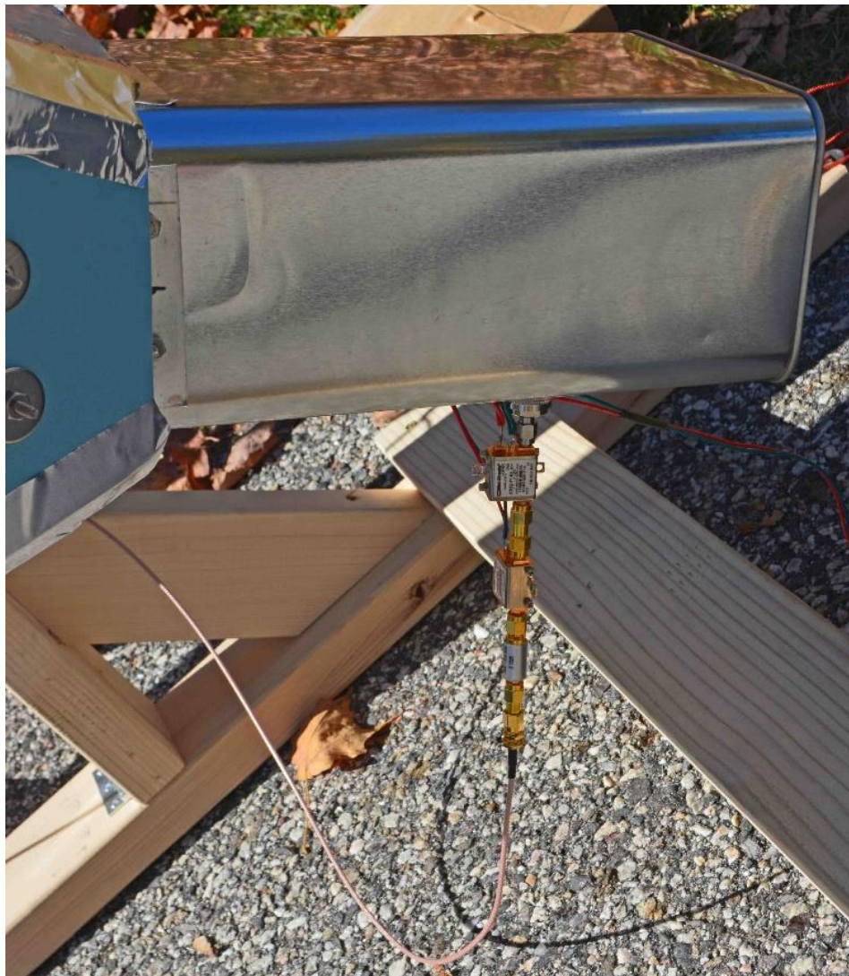
Figure 7: Front-end with LNA's, Bandpass Filter, etc.
